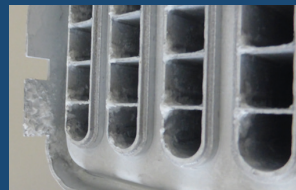
Contamination / residues during the CAB brazing process
